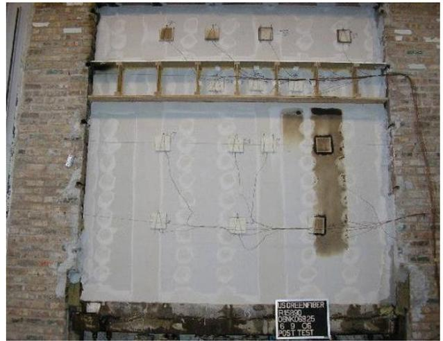
Unexposed Surface – Post-Test Photo
